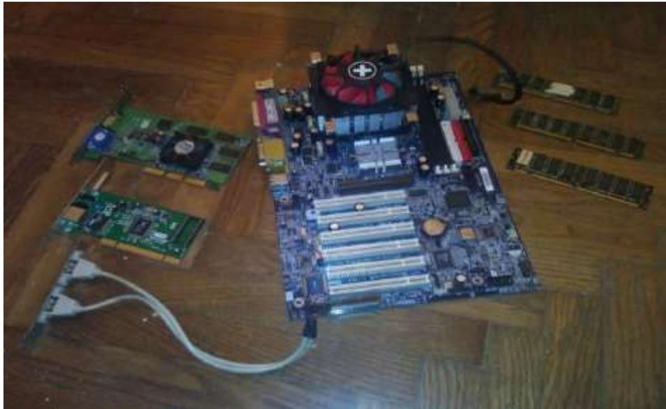
Step 5: Remove the motherboard from the frame of the computer and disconnect the wires to other components.
