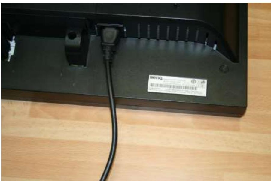
Step 2: Disconnect cable connecting the screen to the computer.
