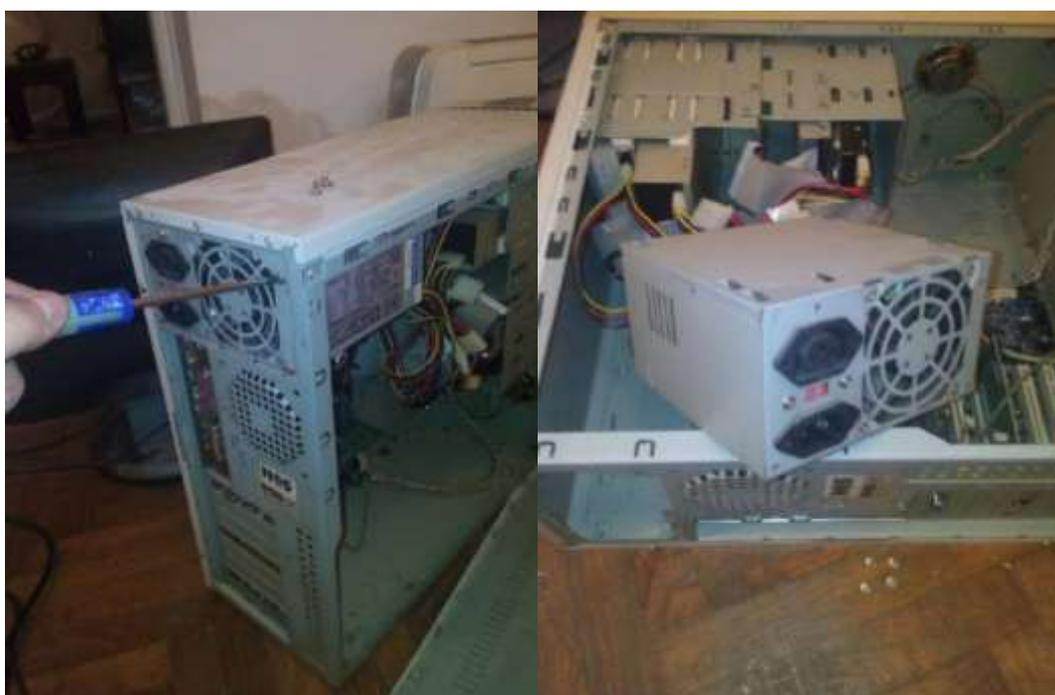
Step 4: Connect the new power supply (assemble in the frame-skeleton of the computer and connect the connection cables with all the construction parts). Attention should be given assembly is the same as before the repair.
