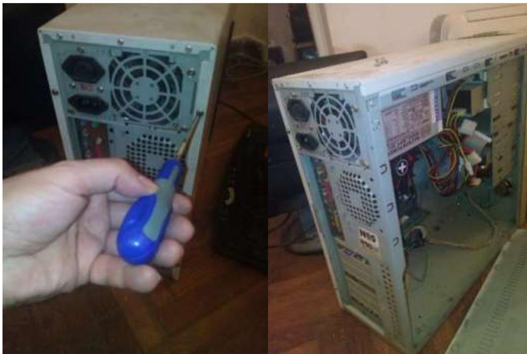
Step 3: Disassemble the power supply from the frame of the computer and disconnect the cables connecting it to other parts.
