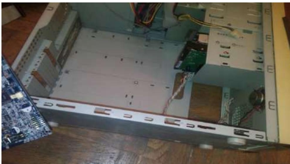
Step 6: Connect the new motherboard to the frame of the computer and connect the wires to other components.
