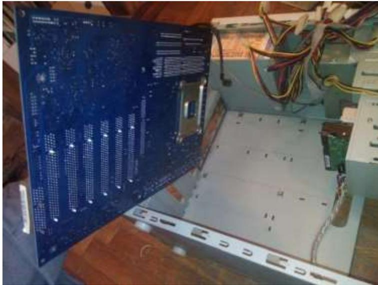
Step 7: Attach the other components (GPU, CPU, network card, hard drives, graphics card, sound card, etc.) to the motherboard. The assembly needs to be the same as before the repair.
