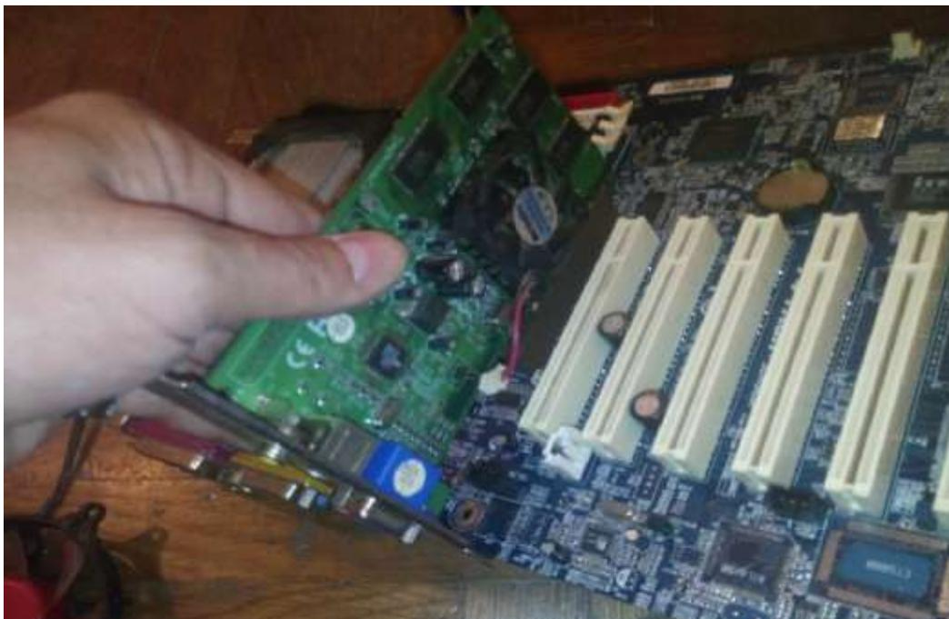
Step 7: Attach the GPU to the socket of the rear part of the computer's frame.
