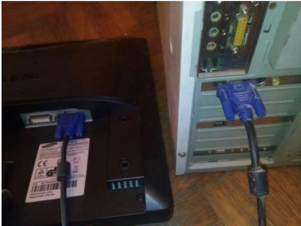
Step 3: Connect the cable from step 2 to the spare screen and the computer.
