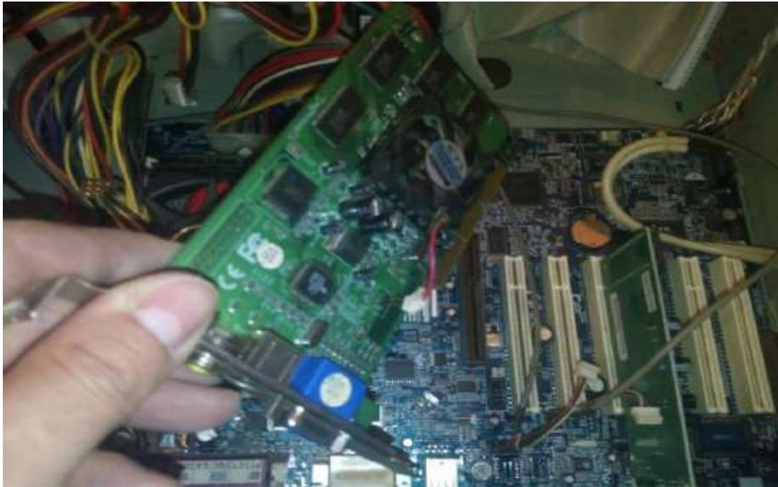
Step 5: Connect the new GPU to the motherboard and reconnect the wires to other parts. The assembly needs to be the same as before the repair.
